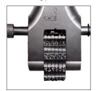
Each 'marking wheel' has 11 faces, with 0 to 9 figures on 10 faces, and one face blank. Stamping is done by a hammer; and the resulting impression is uniform in depth, spacing and alignment of any figure set up. The standard Size Range of ROTARY TYPE NUMERATORS is as follows:
