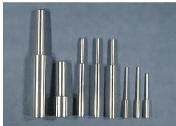
\*Carbide = Tungsten Carbide Hardness approximately 92 Rockwell A, Powdered Metal Hardness 63 – 65 Rockwell C.
